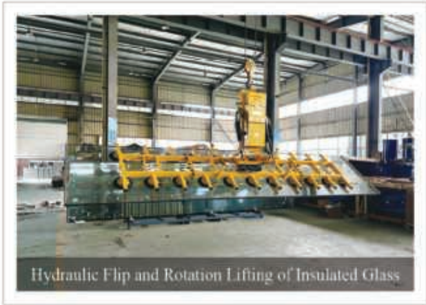
DC-Vacuum Lifter (22 Suckers) FS-YFX2000-22S (2000KG)
