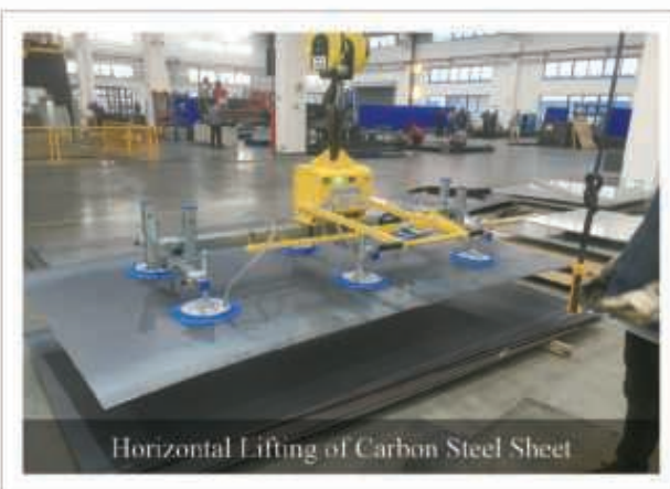
DC-Vacuum Lifter (6 Suckers) FS-BSZ1000-6S (1000KG)
