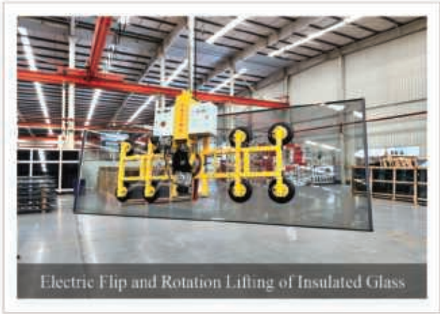
DC-Vacuum Lifter (8 Suckers) FS-DFX800-8S (800KG)
