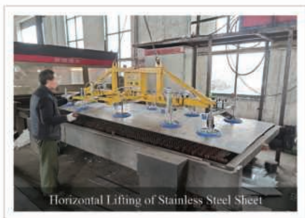
DC-Vacuum Lifter (10 Suckers) FS-BSZ2000-10S (2000KG)
